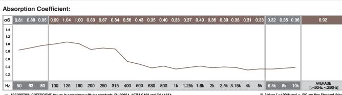
ABSORPTION COEFFICIENT: Values in accordance with the standards: EN 20654, ASTM C423 and EN 11654.
