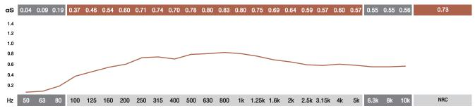
ABSORPTION COEFFICIENT: Values in accordance with the standards: EN 20654, ASTM C423 and EN 11654.
