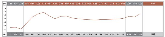
ABSORPTION COEFFICIENT: Values in accordance with the standards: EN 20654, ASTM C423 and EN 11654.
