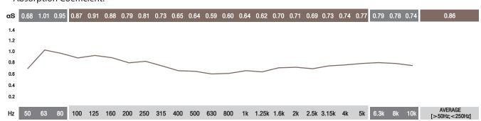
ABSORPTION COEFFICIENT: Values in accordance with the standards: EN 20654, ASTM C423 and EN 11654.
